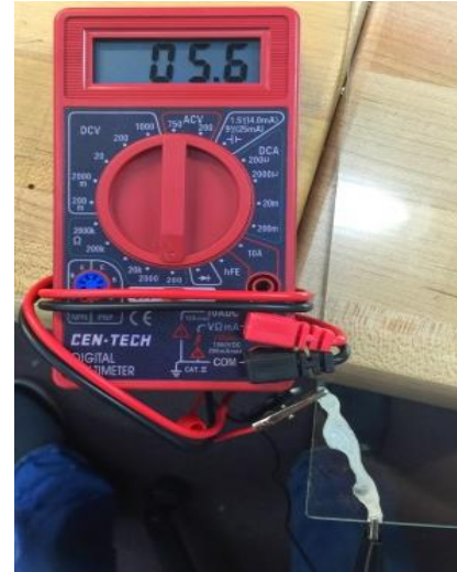
Fig. 4. Test sample of Silver Acetate conductive ink with a multimeter measuring electrical resistance of 5.6 \Omega
