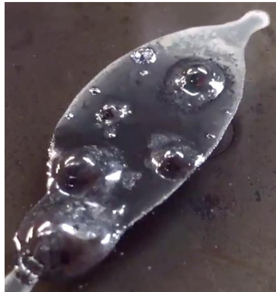
Fig. 2. Test sample of Silver Acetate conductive ink being annealed and fusing into a continuous solid
